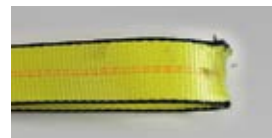
Loop strap damage
