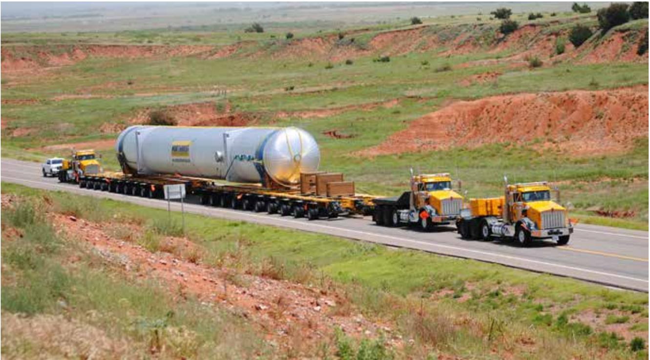
**▲** By using Doleco's textile chains, Oklahoma's Northwest Heavy Haul made securement easier on workers, saved time, and eliminated the potential damage that steel chains would do to the finish on large demethanizer vessels.
