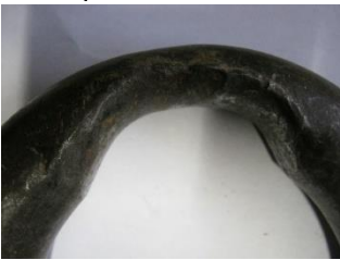
Significantly reduced cross section due to material wear.
