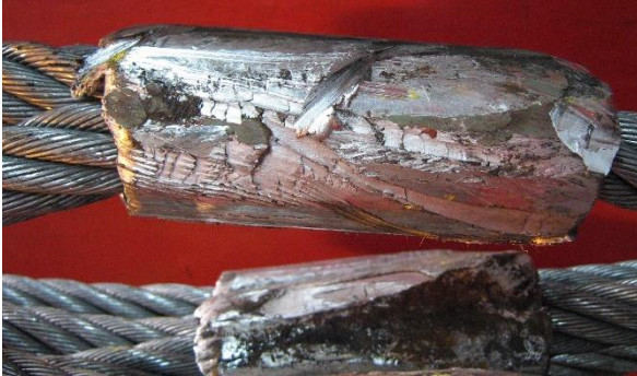
Clearly damaged rope clamps.
