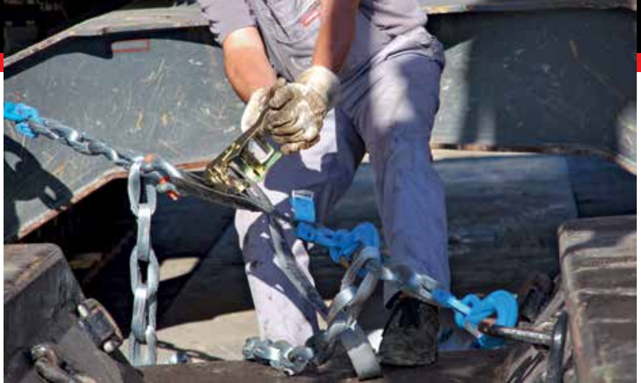
The increased load rating of the textile chains can drastically change how haulers approach securing loads, particularly when DOT regulations come into play regarding the number of chains and where they can be anchored.
